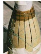
Space the open arc ends evenly. Remember that the spaces at the side of the shroud are each only 1/2 of the space between arc segments. When you are satisfied, tape the arc segments down securely with clear tape (you will need to be able to see through to cut).
