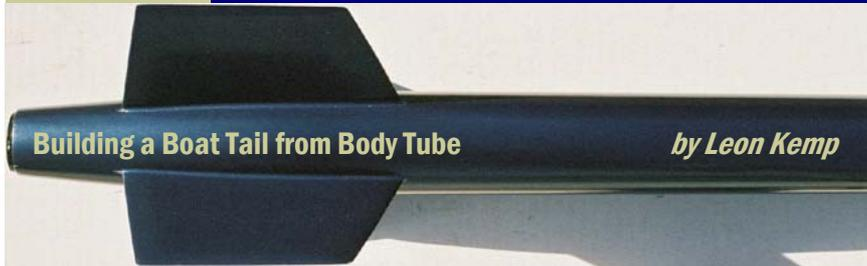
One of the most effective methods of increasing the performance of a rocket is to add a boat tail. Essentially, a boat tail changes the rear of a rocket from a large flat surface with high drag, to smaller (although still flat) surface with lower drag.
